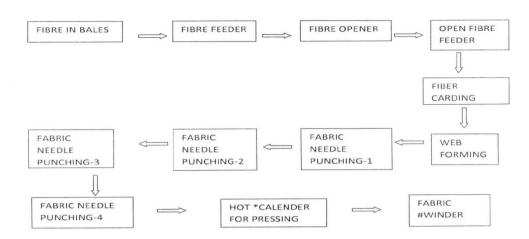
The above flow chart reveals that neither yarn is used as raw material nor process of weaving is undertaken for manufacturing of non woven fabric.
